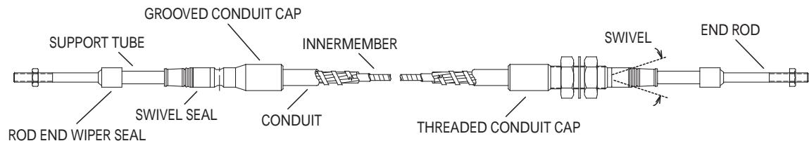
**End Rod and Support Tube** — All standard Cablecraft controls may be ordered with either type 300 stainless steel or protectively plated carbon steel end rods and support tubes. Choose the material to best meet your requirements.
